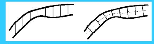
Two approaches to establish areal gridding: (1) on the left, the cells/nodes are stacked vertically, and (2) on the right, the cells/nodes are aligned on lines perpendicular to the bounding surfaces. The first approach, with a universal vertical coordinate, is preferred because of computational simplicity.
