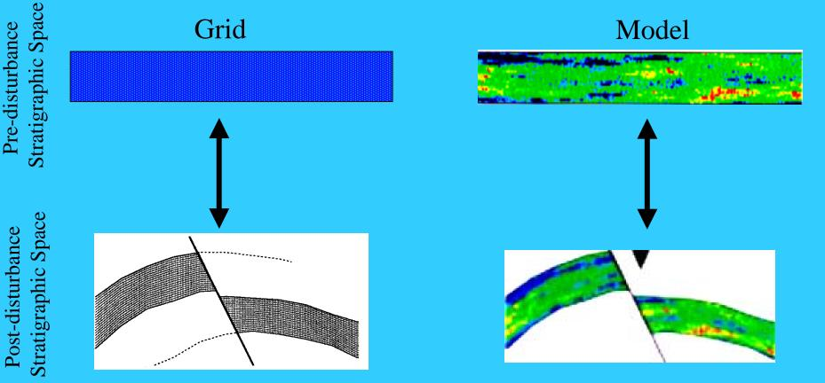
Grid translations may be applied to "remove" faults and tilting in order to work in the predisturbance stratigraphic setting.
